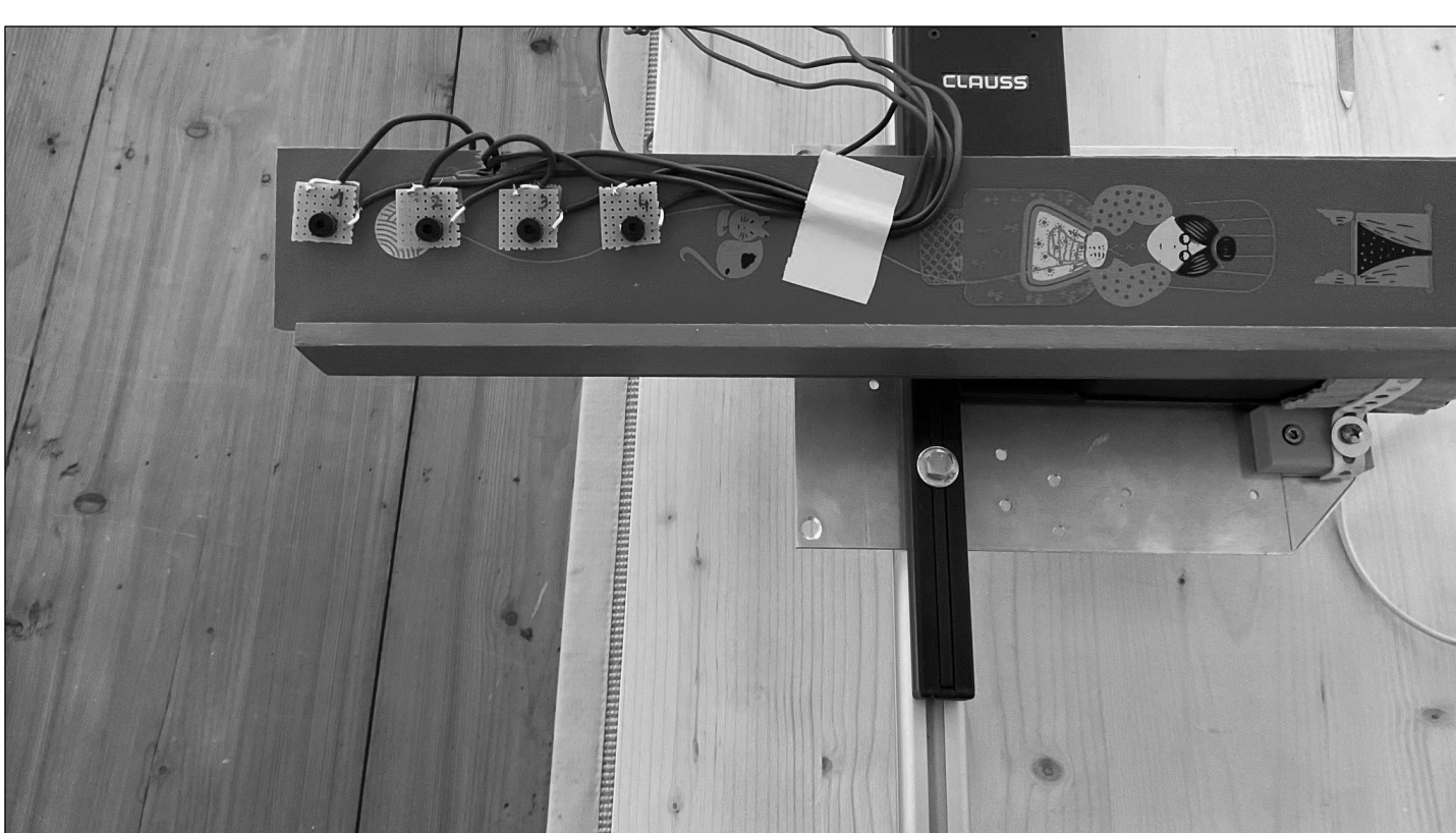
Figure 2: Electronic test model with four microphones and a length of ca. 7.5 cm
